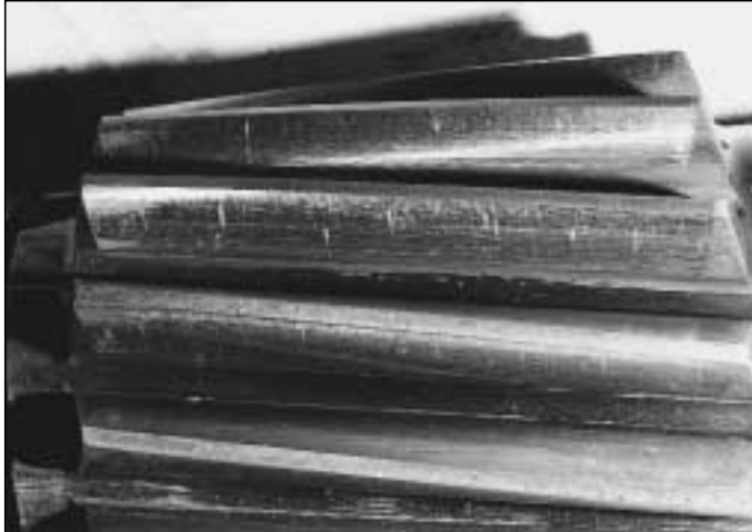
Figure 28 — Adhesion type wear of gear teeth.
