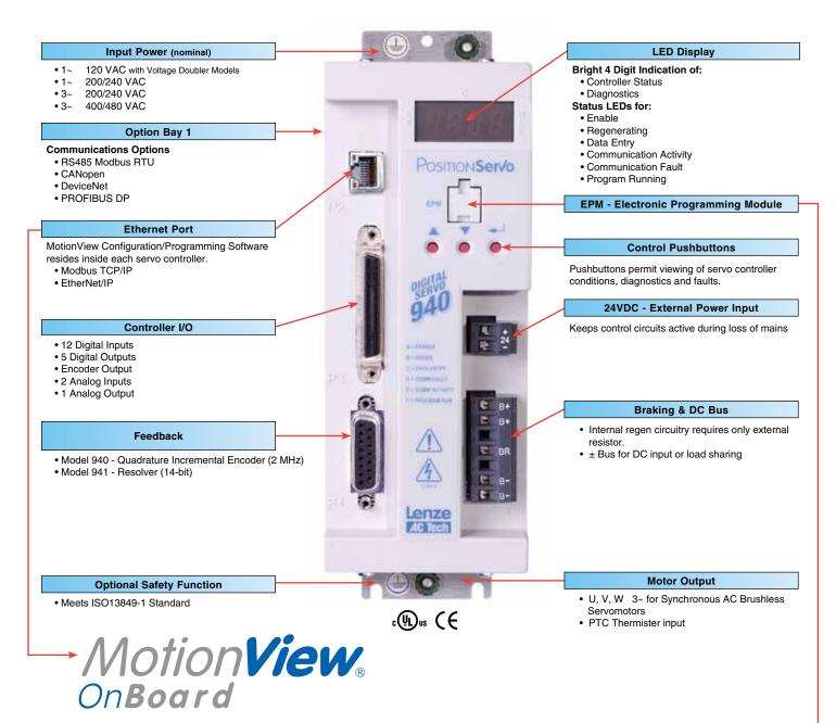
All configuration and programming software is INSIDE the drive. No need for managing firmware or software revisions. It is all done for you.
