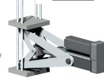
With their high thrust capability, compact size and smooth controlled motion, FT Series actuators are an ideal fit for replacing hydraulics or pneumatics on injection mold toggles. Control improvements from an electromechanical servo system offer less abuse of valuable molds and more consistent performance.
