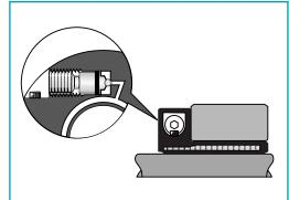
When the pressure screw is tightened to the recommended tightening torque, the steel ball seals against the spherical seat. ETP-TECHNO creates a uniform surface pressure against the shaft and hub.
